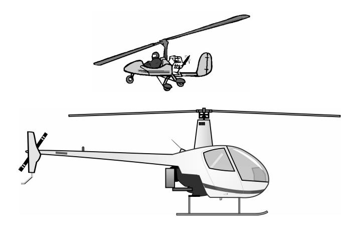
A rotary wing aircraft (rotorcraft) is defined as a heavier than air machine which derives its life from a rotor (or rotors).
