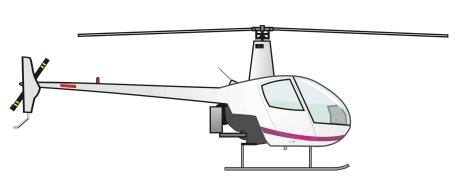
The aircraft relied on its forward speed (provided by either a pusher or puller engine configuration) to produce airflow forces to turn a lift producing horizontal rotor. Today's rotorcraft are practically all helicopters. Unlike the autogyro, helicopters have engine driven horizontal rotors which provide **both** the lift and the propelling forces.
