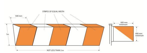
indicate the boundary of an area unfit for the movement of aircraft.
