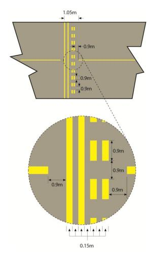
signify the designated visual holding position associated with a runway beyond which no part of a flying machine or vehicle must project in the direction of the runway without permission from the air traffic control unit at the aerodrome during the notified hours of watch of that unit.
