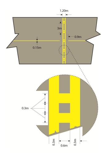
signifies a holding position other than that closest to the runway beyond which no part of a flying machine or vehicle must project in the direction of the runway without permission from the air traffic control unit at the aerodrome during the notified hours of watch of that unit.
