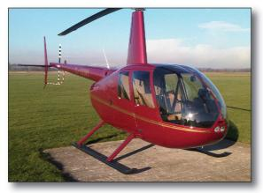
The first version of the helicopter was called the R44 Astro followed by the R44 Raven and R44 Raven II. The Raven had hydraulic cyclic and collective controls as standard while the Astro had an electric cyclic trim and ground-adjustable collective trim with the option of hydraulically assisted controls. The Raven II has a fuel injected engine, the maximum gross weight increased from 2400lbs to 2500lbs, a longer main blade chord, second
